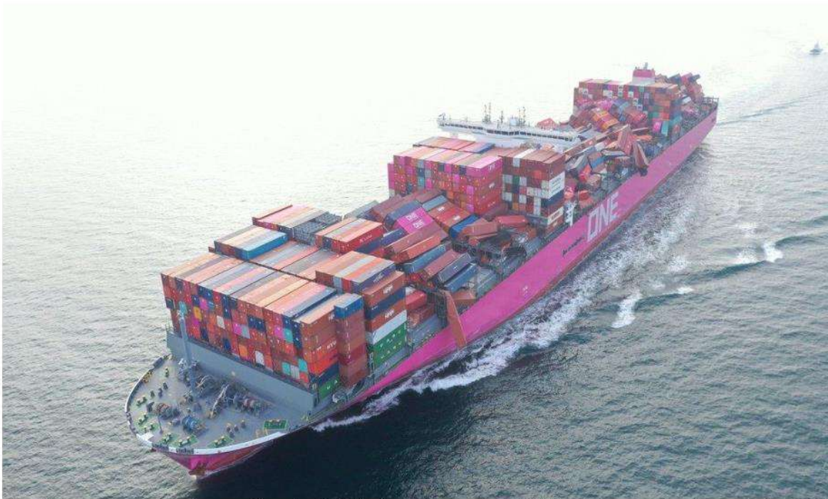
The ONE Apus arrives in Kobe, Japan on December 8, 2020, after losing an estimated 1,816 containers overboard approximately 1,600 nautical miles northwest of Hawaii, USA. Photo courtesy W K Webster and Co.
